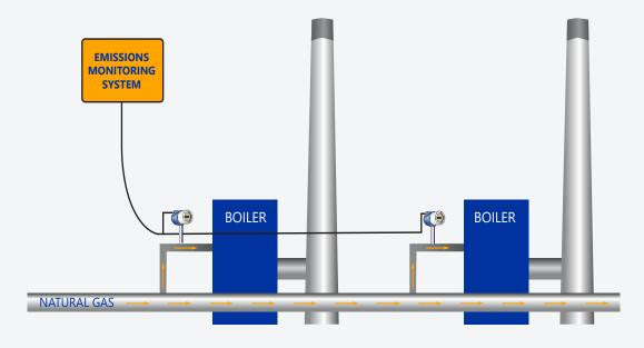
Natural gas measurement by totalizing fuel flow (TFF) meters used in an emissions monitoring system to calculate total emissions.
