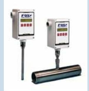
The Fox Model FT2 Thermal Gas Mass Flowmeter and Temperature Transmitter measures two important process variables with one rugged instrument. The Model FT2 measures gas flow rate in standard units without the need for temperature or pressure compensation. It provides isolated 4 to 20mA and pulse outputs for flow rate, and a 4 to 20mA output for process gas temperature. The pulse is normally used for totalization. [Learn More](#)
