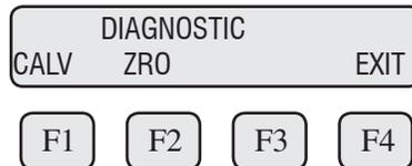
Press **ZRO (F2)** to choose the type of Zero CAL-CHECK™ test.
