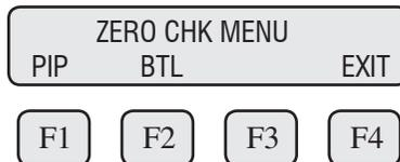
Press **BTL (F2)** to choose to perform the test out of the pipe. The display will show:
