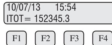
The Date & Time is displayed on line 1 and the interval total on line 2. The interval total is based on the flow units selected in the meter (total mass flow or total volumetric flow).
