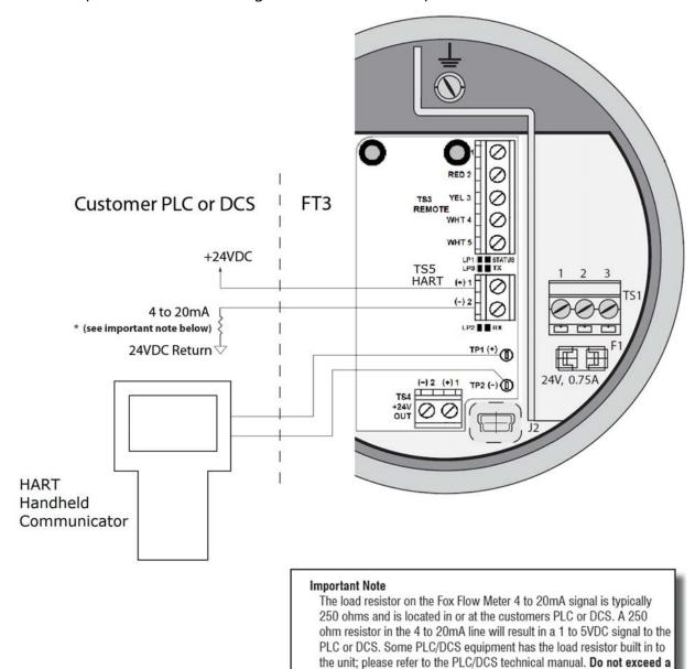
600 ohm load on the Fox Flow Meter 4 to 20mA signal.
